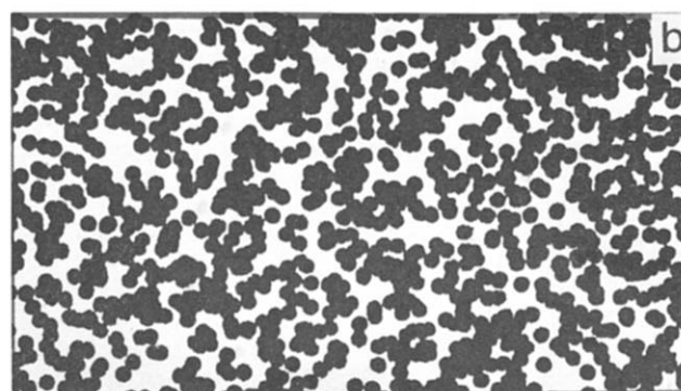
Figure 8 (a) S mapping of the specimen in Figure 7. (b) Modified S mapping: dots in (a) are widened to circles of 0.25 µm diameter
